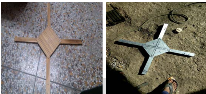
Figure1: (a). Prototype model of frame made by wood (b). Aluminum Frame.
